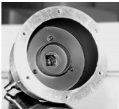
Figure 18: Dummy FPA with the PM photocathode in the focal plane.
