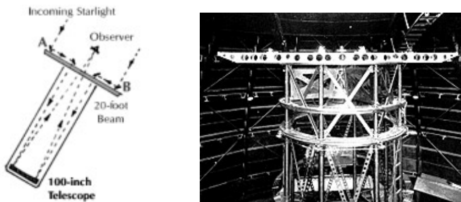
Figure 1.5: Left: Optical layout of a rudimentary Michelson stellar interferometer, as used by Michelson (1919). Right: Photograph of the 2.5-m Hooker telescope surmounted by a 6-m metal beam. Taken from the Space Interferometry Mission (SIM) web-site.
